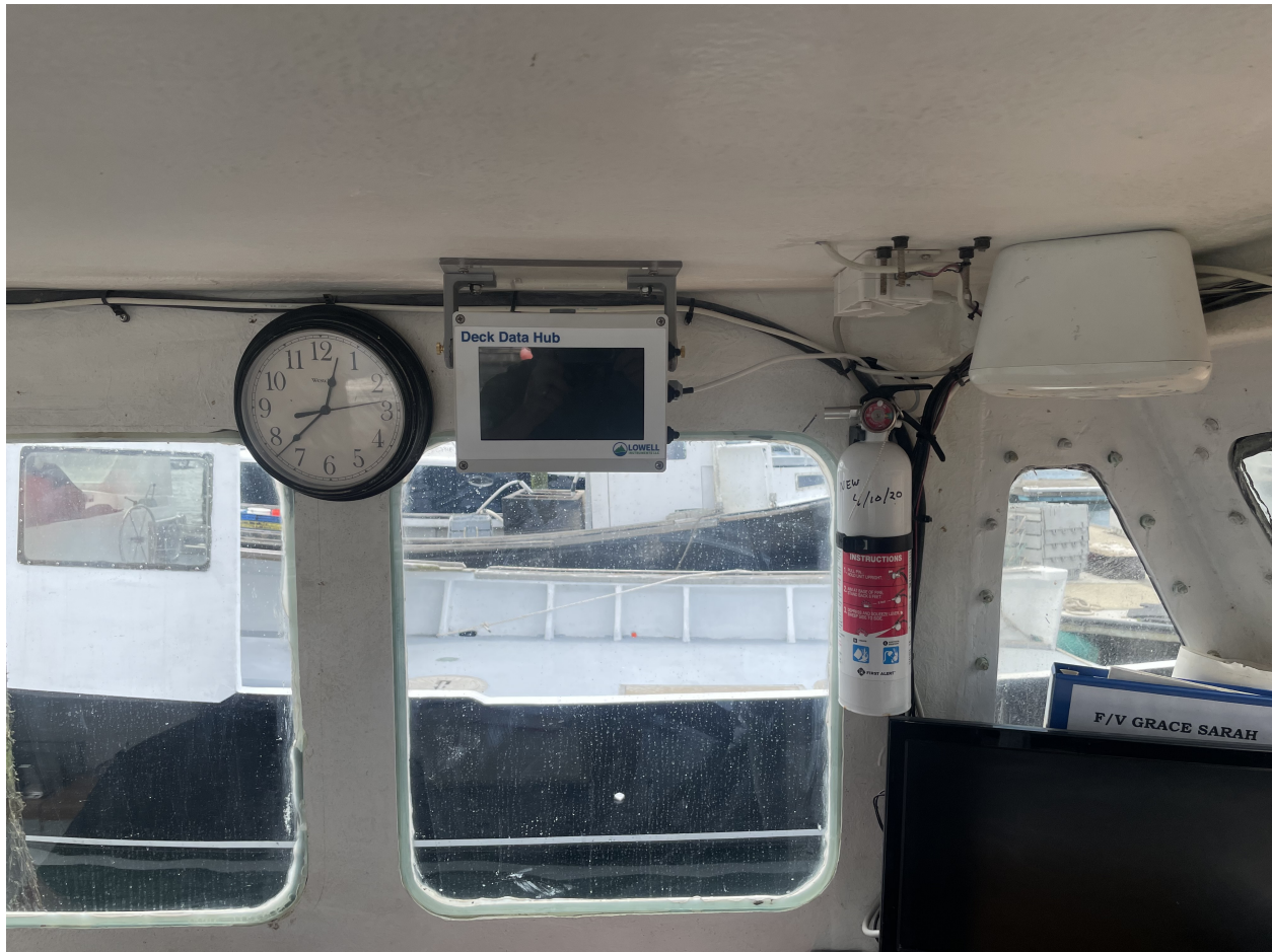
Figure 4 – A Deck Data Hub (Lowell Instruments LLC., Falmouth, MA) allows fishermen to see the dissolved oxygen and temperature data collected on their gear and transmits data back to scientists at DMF and NOAA in near real time
