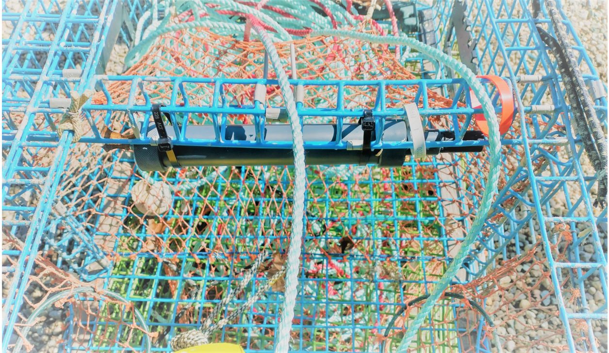
Figure 3 – A dissolved oxygen probe installed on a lobster trap
