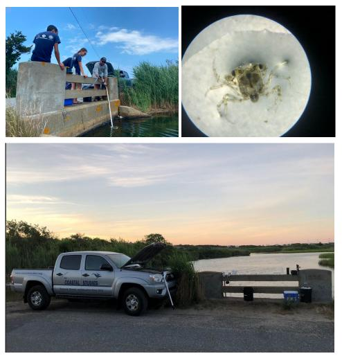
The CCS Toyota Tacoma often served as a mobile plankton laboratory this summer. A pump sampler designed and built by Marine Fisheries Research Director Owen Nichols operated off the truck's battery, filtering plankton from hundreds of gallons of water.
